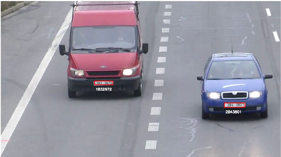
Figure 5.7: An example of the video output mode showing the bounding boxes and license plate texts.
