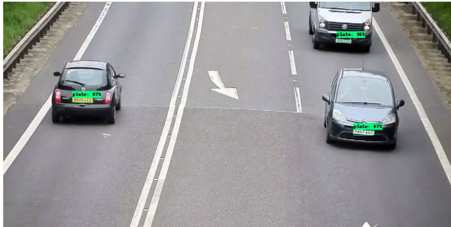
Figure 5.4: The visualized output of the detector — predicted bounding boxes with their respective confidences.
