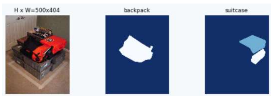
Figure 9 - Masks created with polygonal labels for training a Mask R-CNN network
