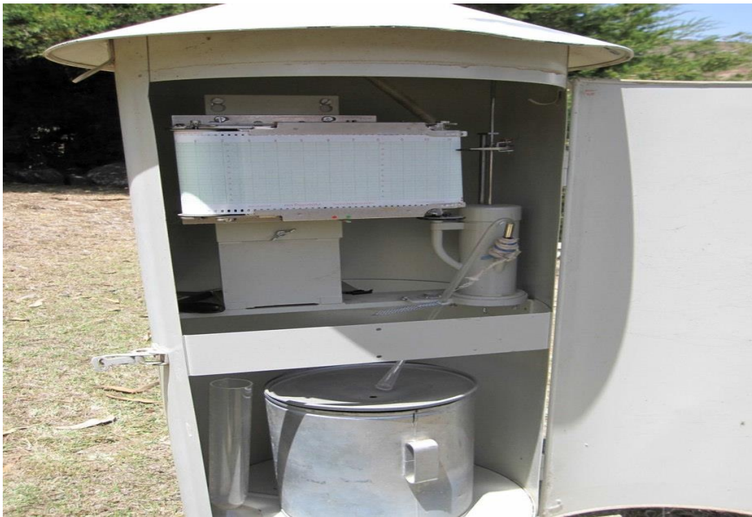
Figure 6: Automatic rain gauge installed at the site's meteorological station (Source: Author)
