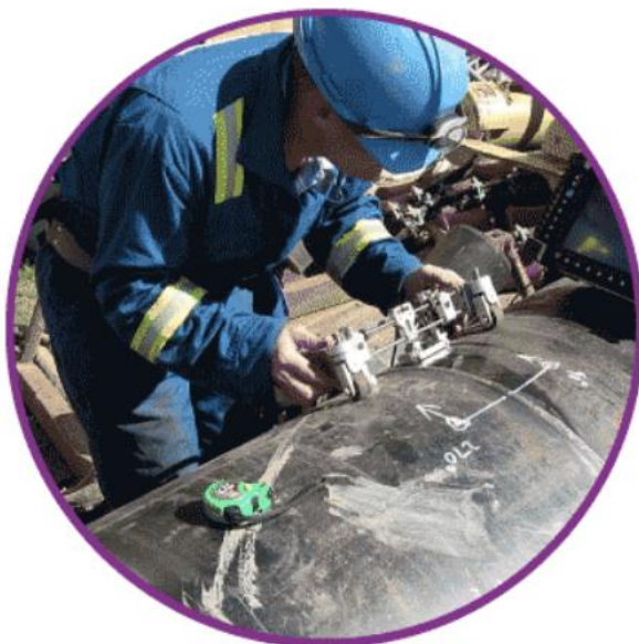
Figure 11: Cracks detection in metallic components using ultrasound
