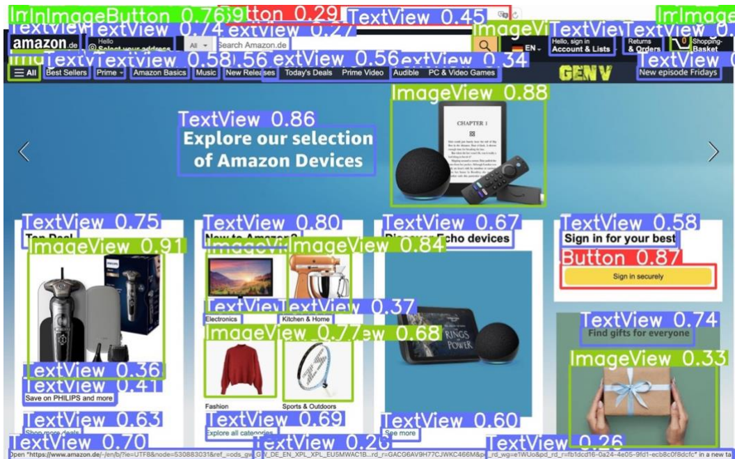
Figure 15. Result of detection UI elements. YOLOv8s.
