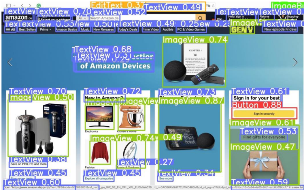
Figure 14. Result of detection UI elements. YOLOv8n.
