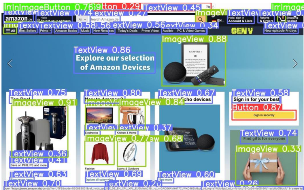
Figure 15. Result of detection UI elements. YOLOv8s.
