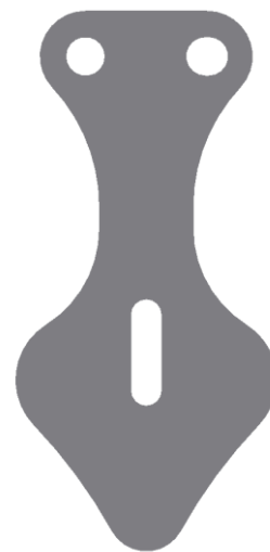
Figure 10.8 Second suction valve design
