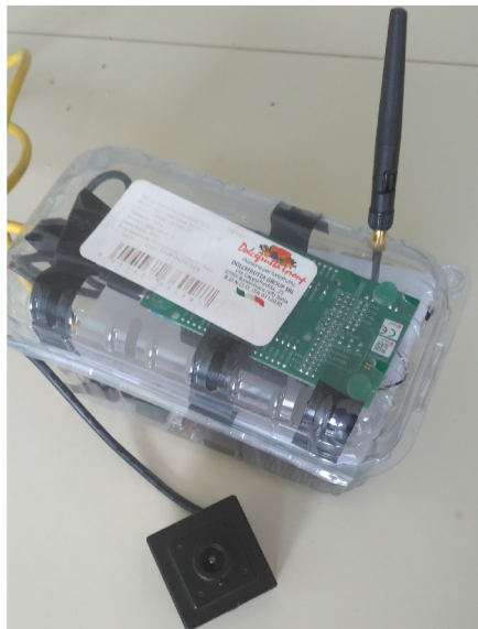
Fig. 3.9: Device enclosed in a plastic box
