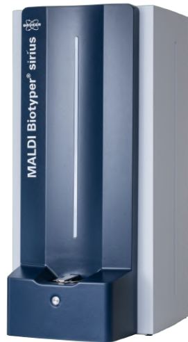
Figure 2.5: The MBT Biotyper – an instrument for classifying microbial species based on the MALDI-TOF technique. Samples for analysis are fed into the machine on prepared MALDI target plates.
