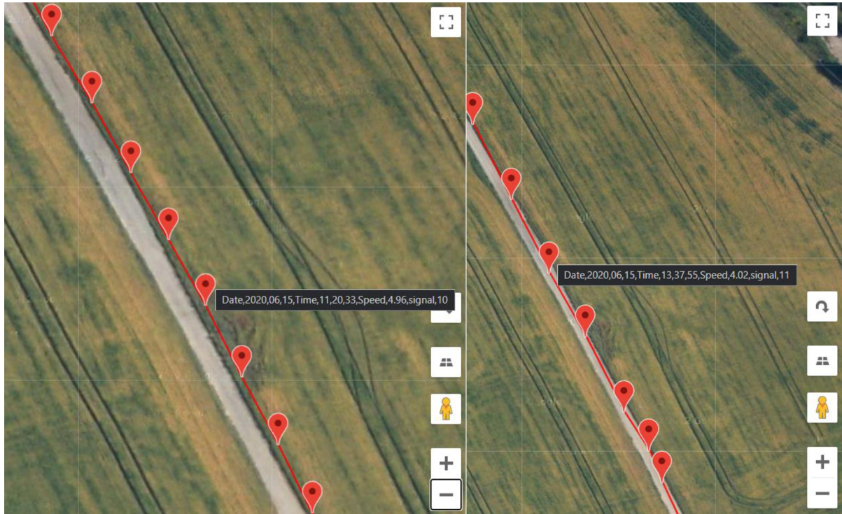
Figure 4.3 passive (left) VS active (right) antennas
