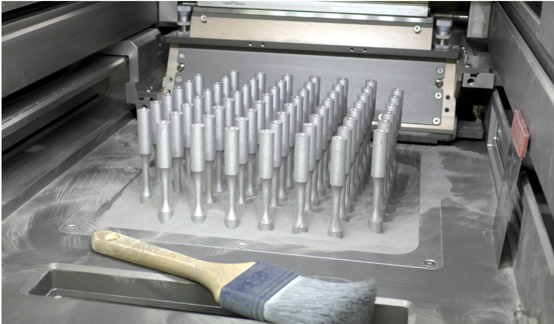
Figure 6.2: ASTM E606 specimens after print on SLM 280 HL
