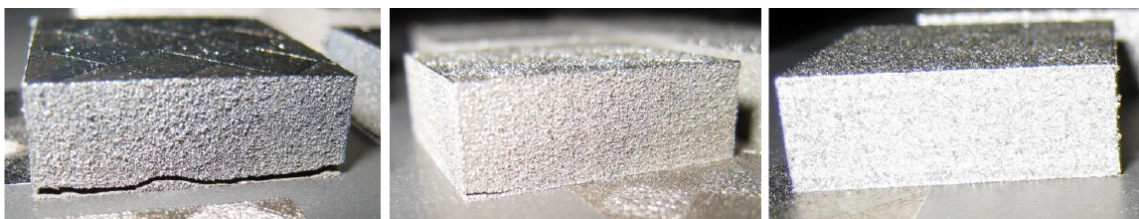
Figure 2.10: M2hss part produced with pre-heating module with 90 °C (left), 150 °C (middle), 200 °C (right) [8]
