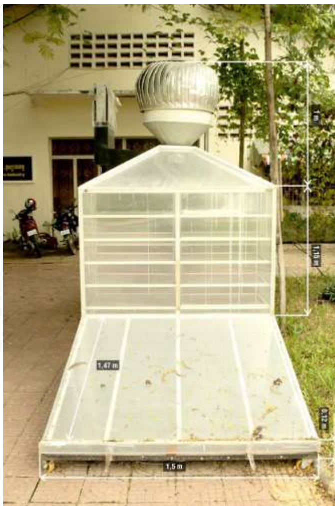
Figure 3.5 Photograph of a natural convection solar dryer
