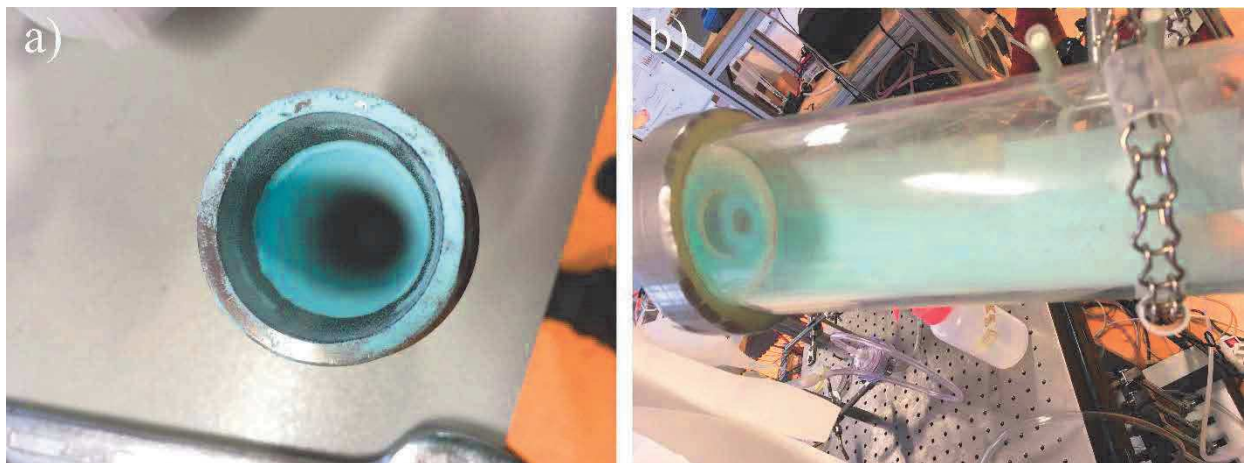
Figure 43 Particle deposition throughout the experimental setup; a) the expansion cone inside the SSPD, b) the dilutor
