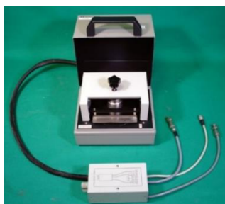
Obr. 14 Agilent 16008B Resistivity Cell
