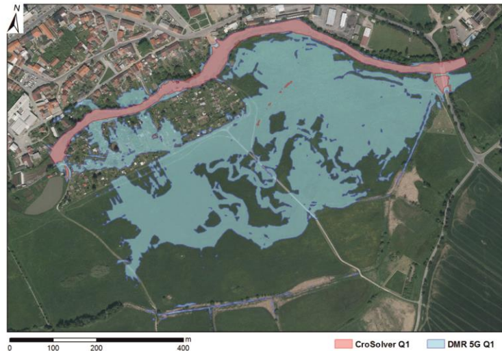
Fig. 23 Comparison of inundation areas at discharge Q_1 in the Úhlava R. locality
