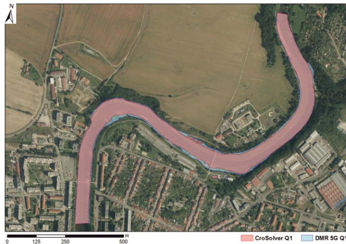
Fig. 15 Comparison of inundation area at discharge Q_1 in the Otava locality
