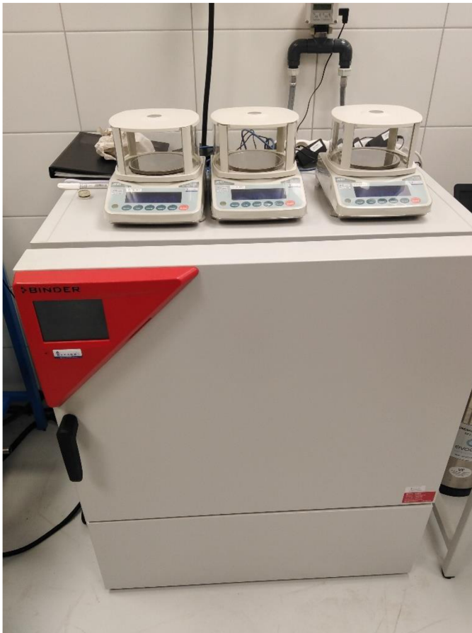
Fig 6: Oven dryer used for the mango drying experiments (Author 2023)
