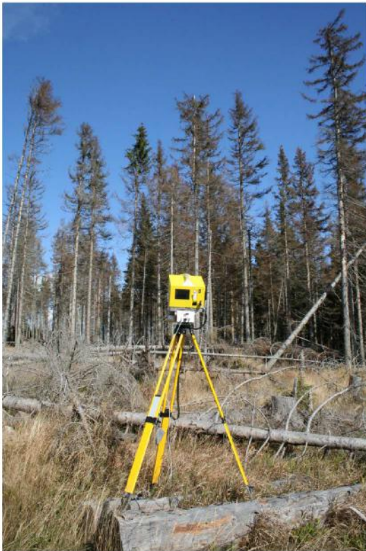
Figure 3.3: OPTECH Ilris-36D terrestrial laser scanner.
