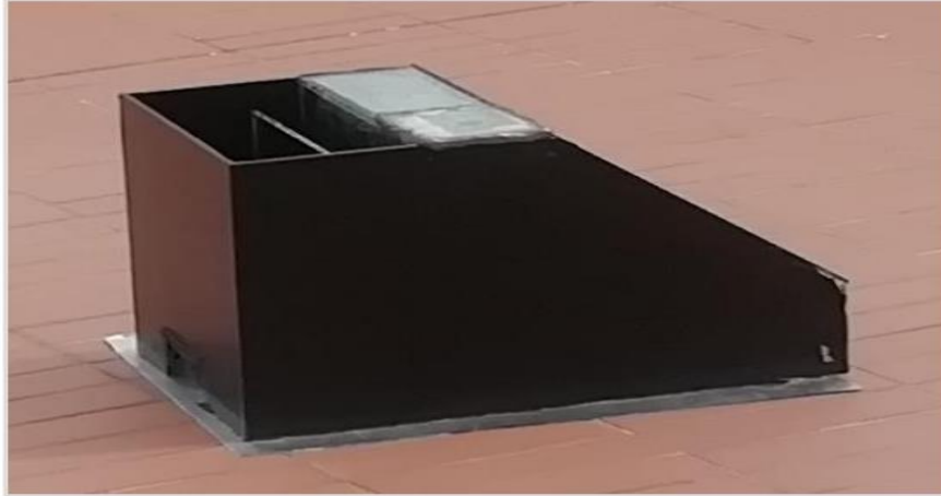
Figure 7 Solar Still Side. The solar still is 0.50 m long and 0.30 m wide, respectively. It is covered with black adhesive paper to improve the absorptivity of solar radiation and increase the internal heat of the solar still.[29]
