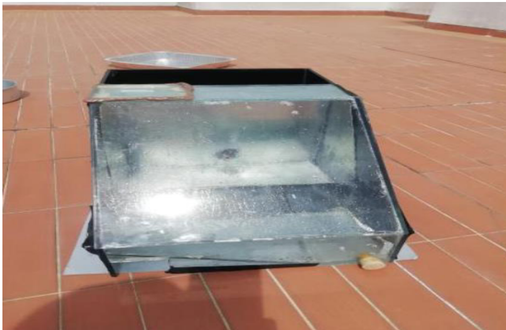
Figure 8 Solar Still used in field trail front view. The wall of the solar still ere build in glass with a thickness of 5 mm and the water basin was in metal. [29]
