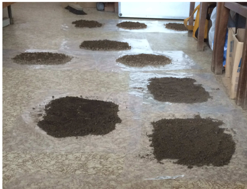
Figure 10. Chernozem and Luvisol samples are left to dry after being sprayed on plastic sheets before being packed into the Kopecky rings.
