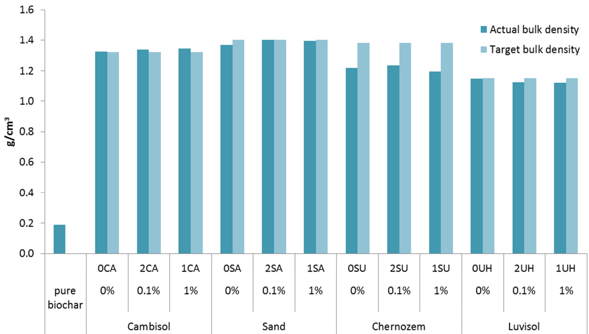
Figure 15. Actual and target bulk densities in all tested variants of biochar admixtures.
