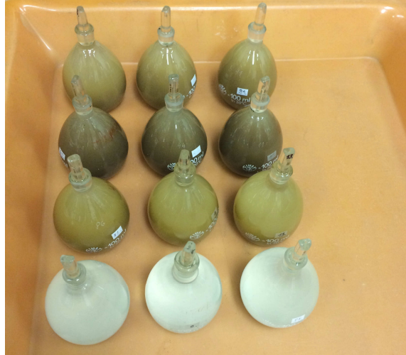
Figure 14. Pycnometers with all soil samples (photo taken in laboratory).
