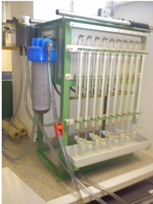
Figure 10 - Permeameter for measurements of saturated hydraulic conductivity (Author's photo)
