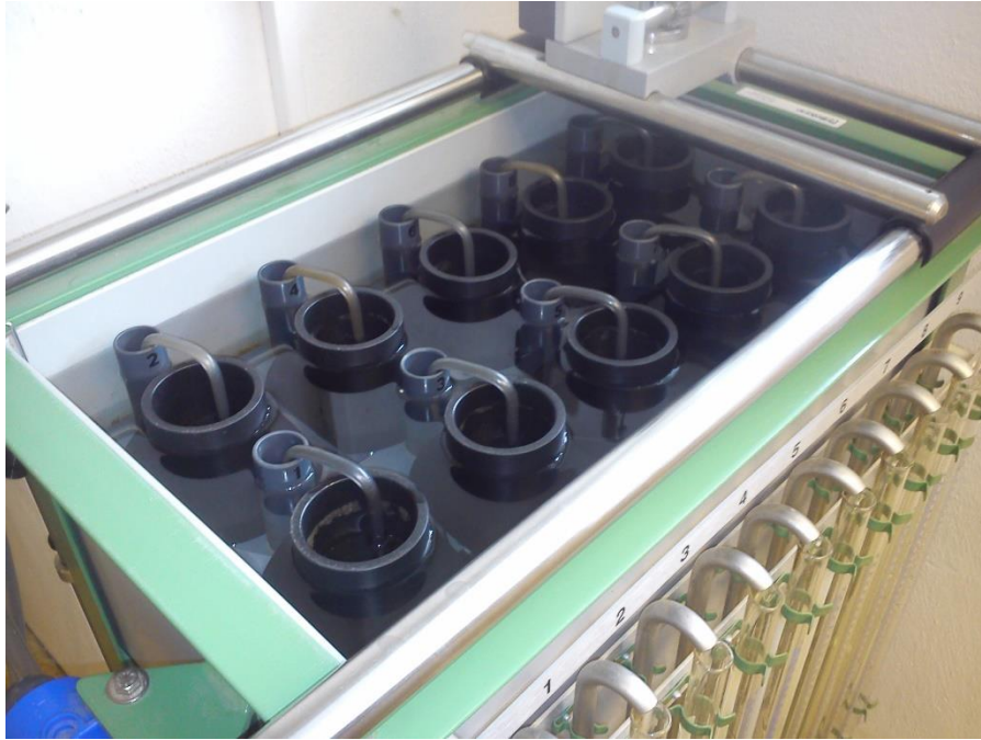
Figure 11 - Samples during measurements of saturated hydraulic conductivity in permeameter (Author's photo)
