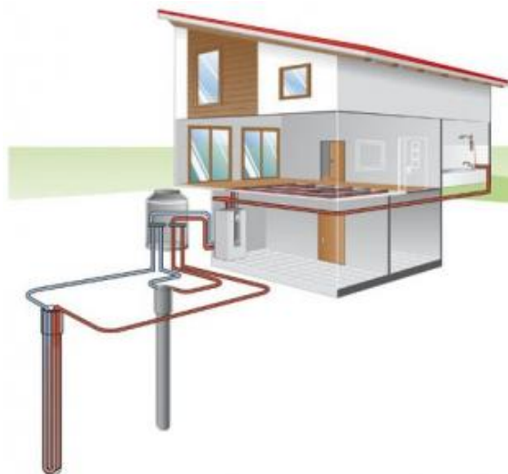
Picture 2.15. – Vertical boreholes solution [16]
