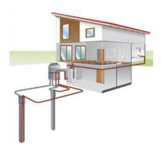
Picture 2.15. – Vertical boreholes solution [16]
