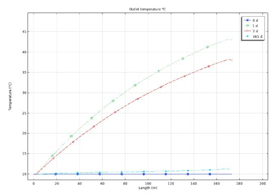
Chart 4.9. – Outlet temperature for inconstant soil temperature
