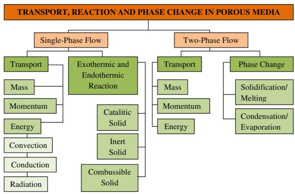
Picture 4.7. – Aspects of treatment of transport, reaction and phase change in porous media [24]
