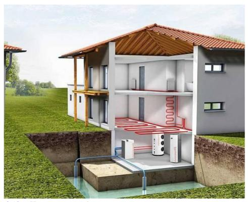
Picture 2.12. – Heat pump water/water [36]
