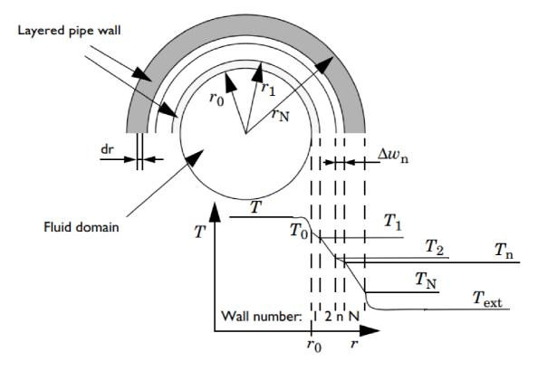
Picture 3.2. – Temperature distribution across the pipe wall [34]
