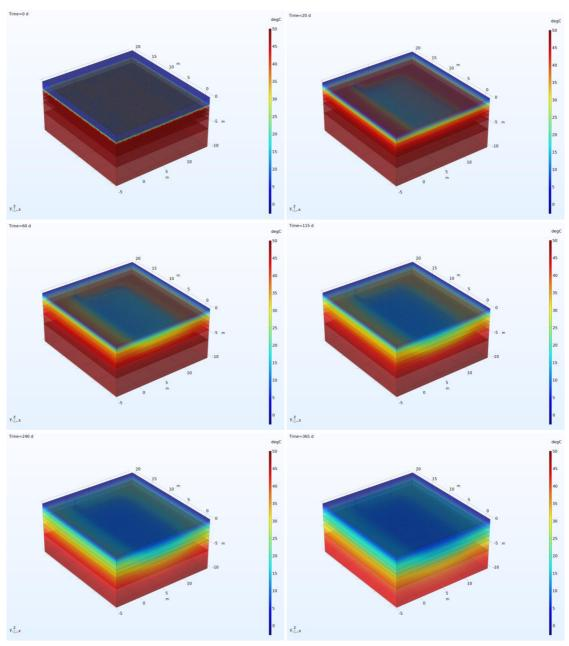
Picture 4.13. – Image sequences of subsurface symmetrical cooling
