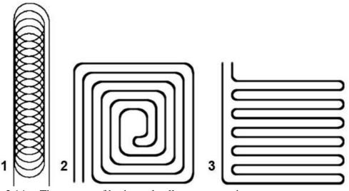
Picture 2.14. – Three types of horizontal collector connection [20]
