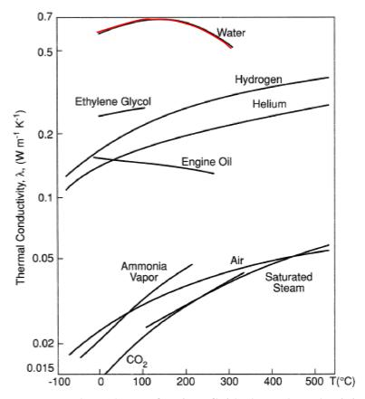
Chart 4.6. – Temperature dependence of various fluids thermal conductivity [10]
