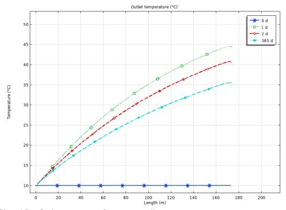
Chart 4.7. – Outlet temperature for constant soil temperature
