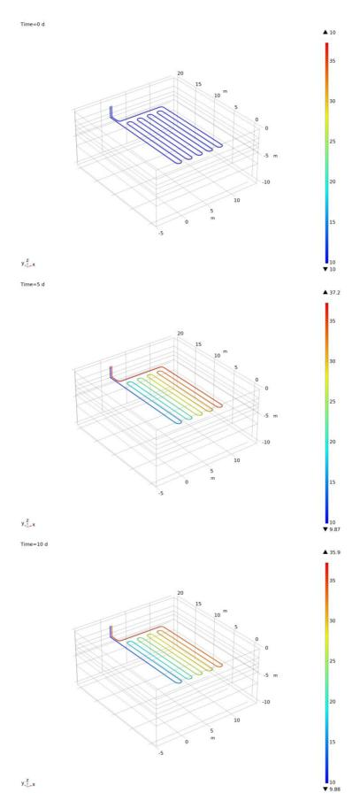
Picture 4.12. – GHE temperature profile for the constant soil temperature
