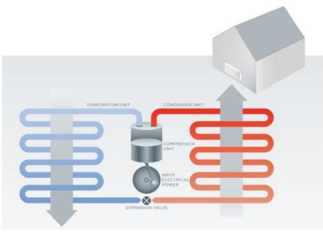
Picture 2.10. – Basic principle of heat pump [18]
