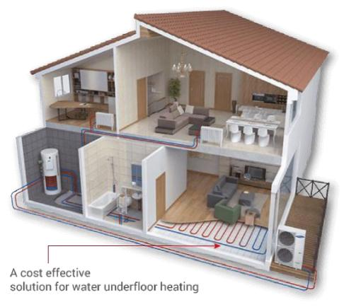
Picture 2.11. – Possibilities of heat pump air/water use [3]
