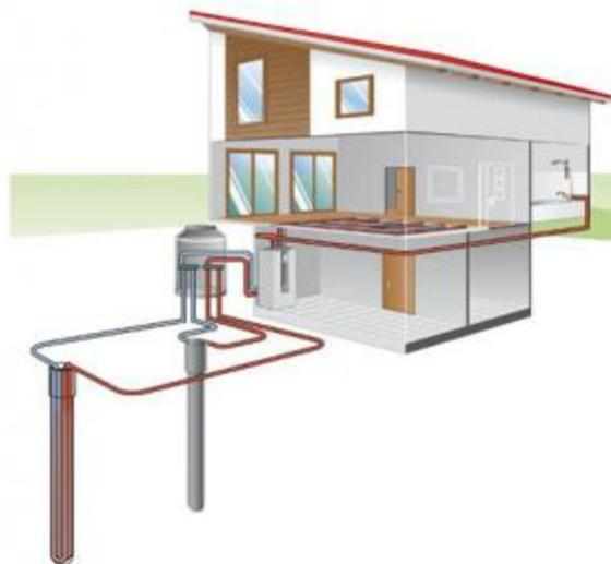
Picture 2.15. – Vertical boreholes solution [16]
