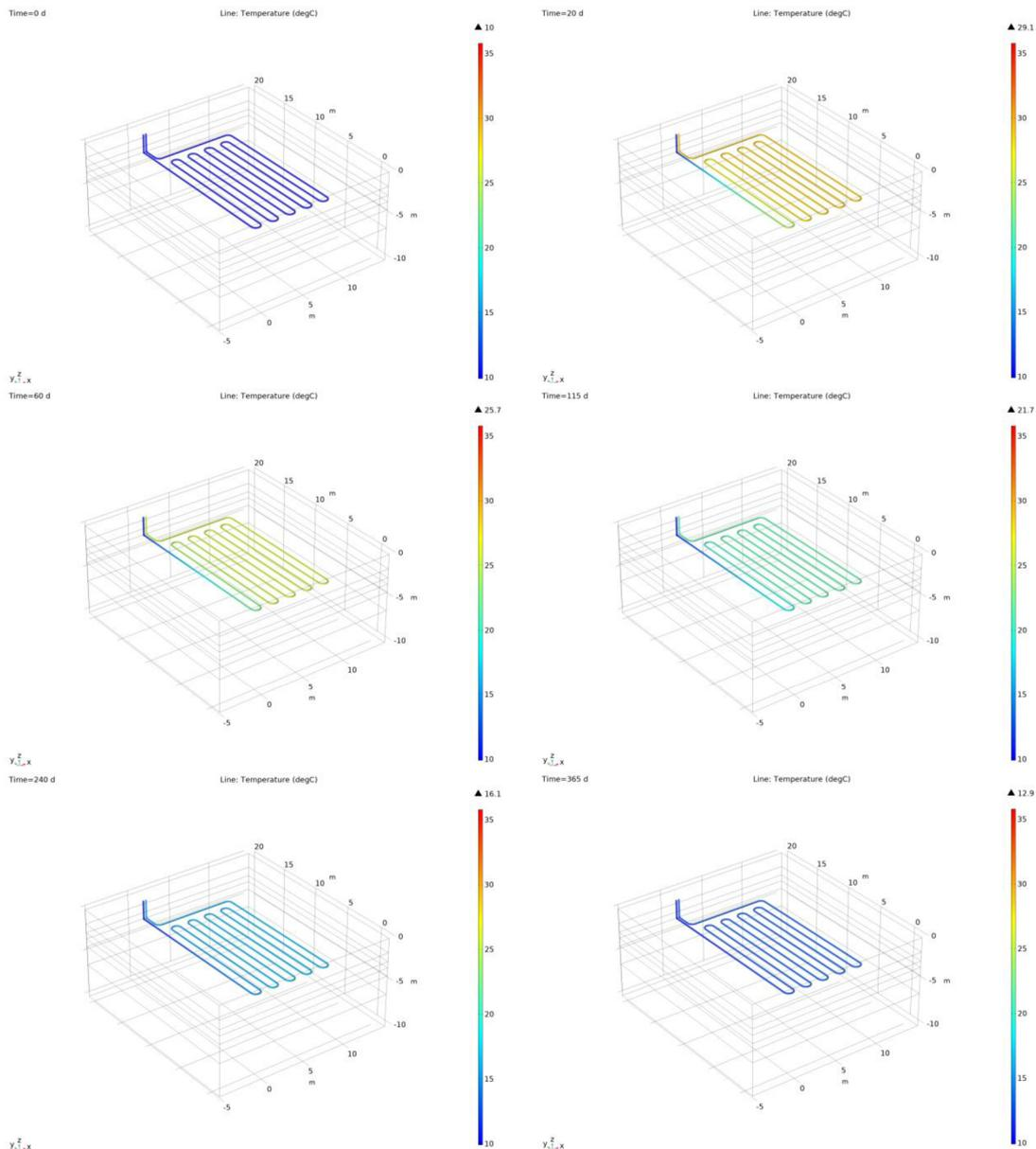
Picture 4.18. - GHE temperature distribution with groundwater flow
