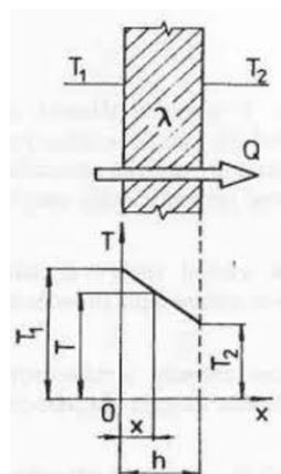
Picture 2.6. – Heat conduction by flat wall [7]
