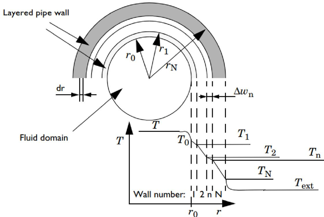
Picture 3.2. – Temperature distribution across the pipe wall [34]
