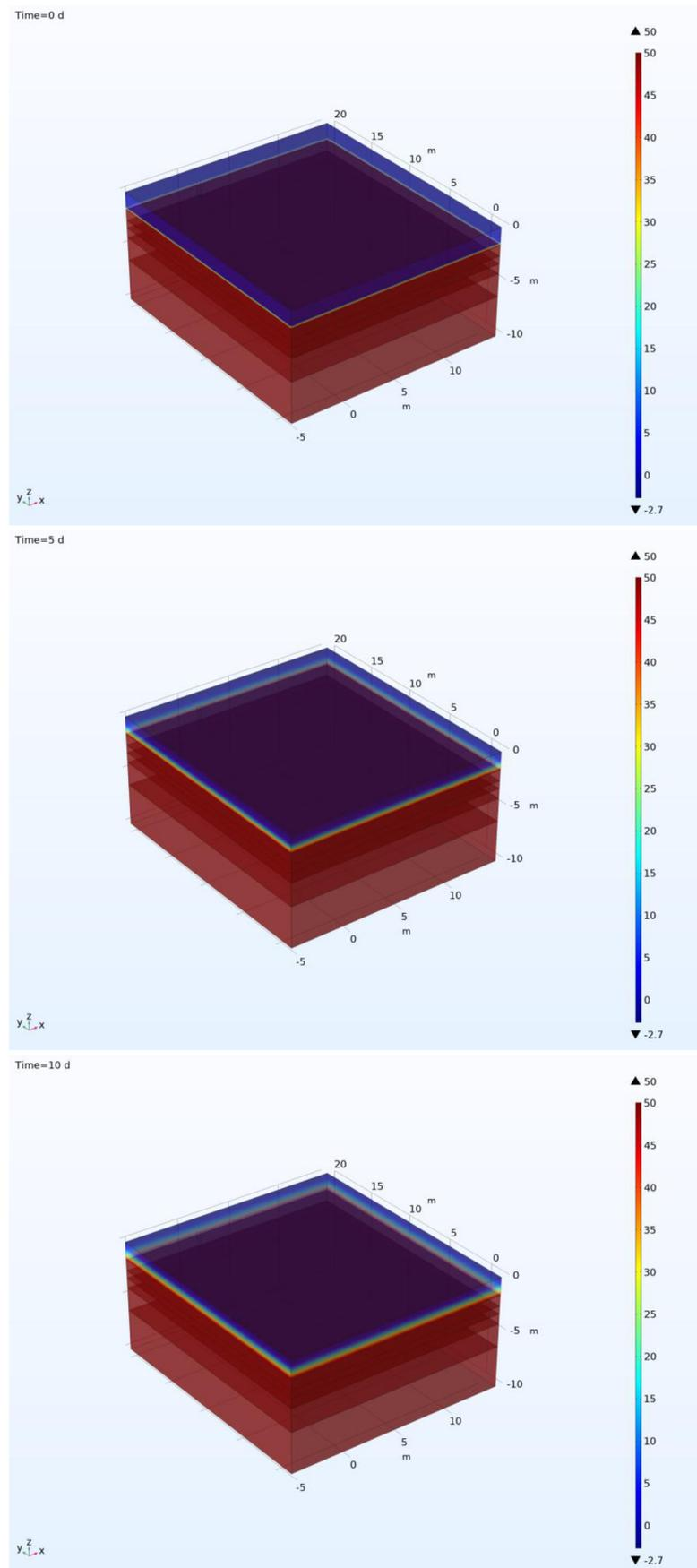
Picture 4.11. – Dynamic behaviour of the subsoil at initial state, 5<sup>th</sup> day and 10<sup>th</sup> day of operation
