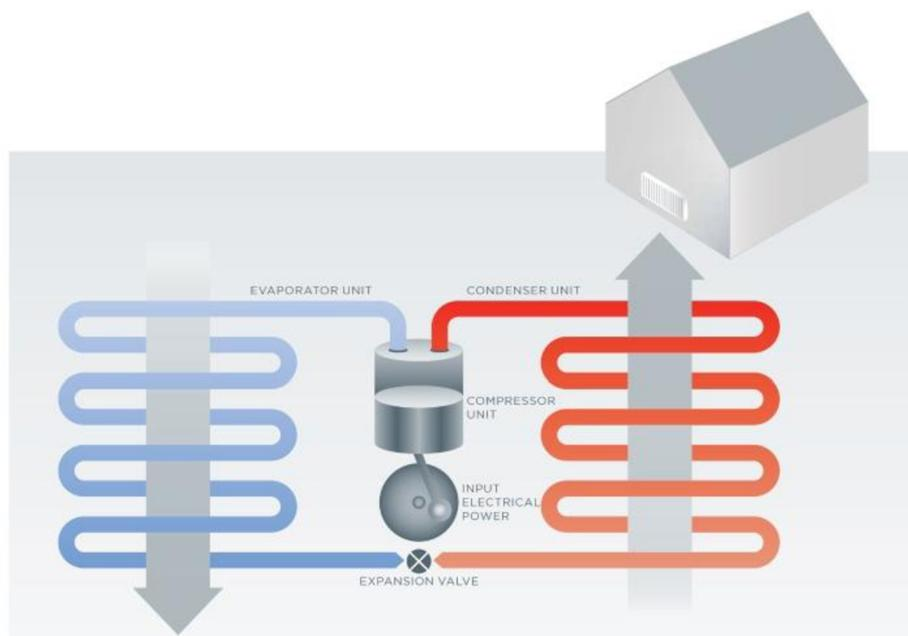
Picture 2.10. – Basic principle of heat pump [18]
