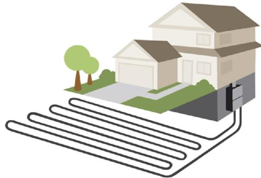
Picture 2.13. – Horizontal ground source heat pump [42],
