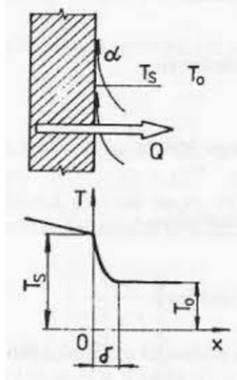
Picture 2.7. – Heat transfer by convection [7]
