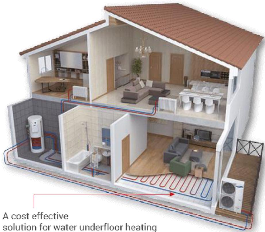
Picture 2.11. – Possibilities of heat pump air/water use [3]
