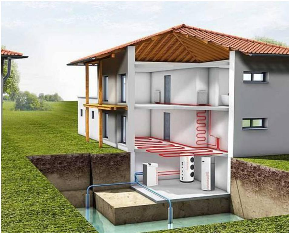
Picture 2.12. – Heat pump water/water [36]
