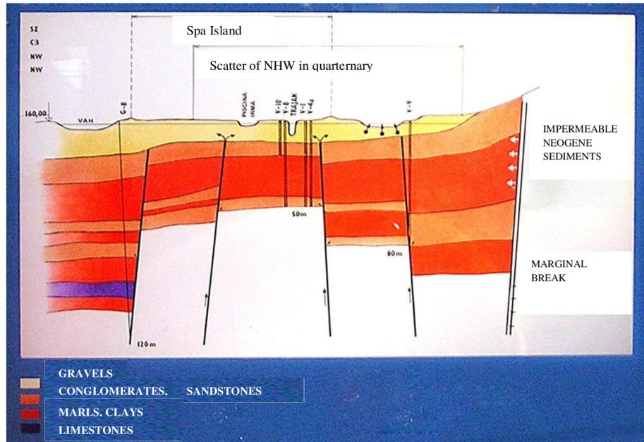
Picture 4.3. – Scheme of spring area construction [Source: Archive of SLKP a.s.]
