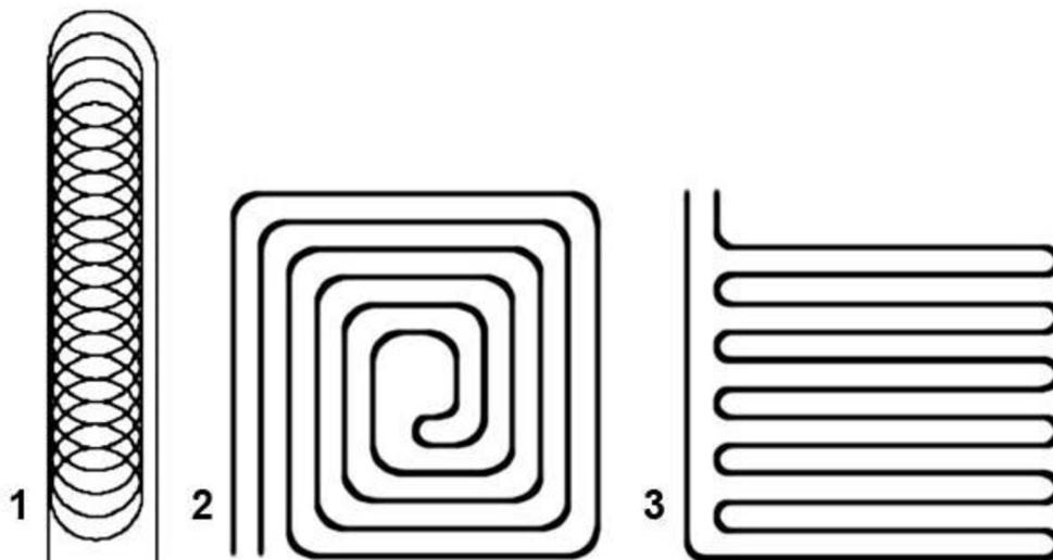
Picture 2.14. – Three types of horizontal collector connection [20]
