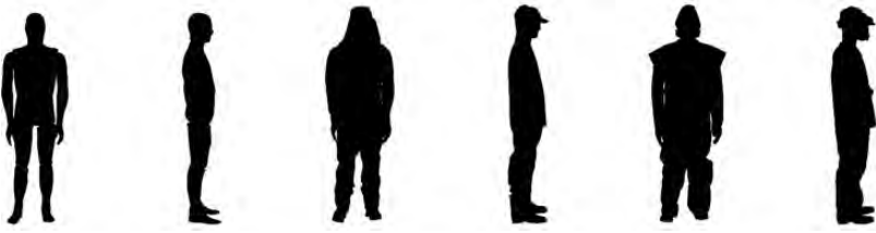
Figure 2. Edited photos of the nude manikin, SC – the sugarcane cutter's outfit, and PS – the pesticide sprayer's outfit, which were used to count black pixels for the clothing area factor ( f_{cl} ) calculation.
