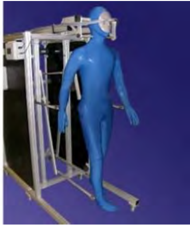
Figure 3: Sweating 'Newton' type manikin with water supply through pores made by Thermetrics, Seattle, USA
