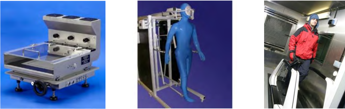
Figure 1: Sweating guarded hot plates SGHP-8.2 and Sweating thermal manikin Newton from Thermetrics, Advanced Thermal Measurement Technology, Seattle, USA; test person from Santra Technology, UK website.
