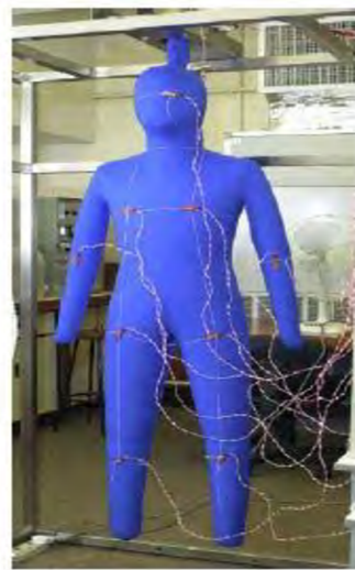
Figure 2: Sweating manikin “Walter” from Hong Kong Polytechnic University with GORE-TEX skin, taken from (Fan and Chen 2002)
