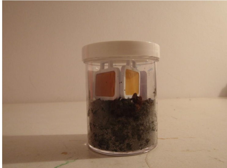
Figure 3.4: Detail of CO 2 and NH 3 paddles during compost maturity tests.
