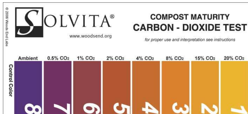
Figure 3.5: Color key for compost maturity according to carbon dioxide. Source: Solvita (2013)
