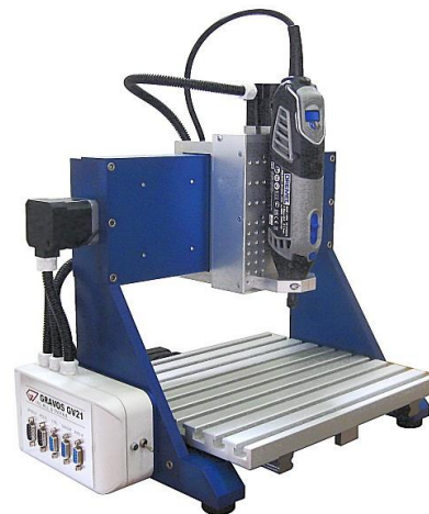
Obr. 7 – Frézka GV 21 2A [14]
