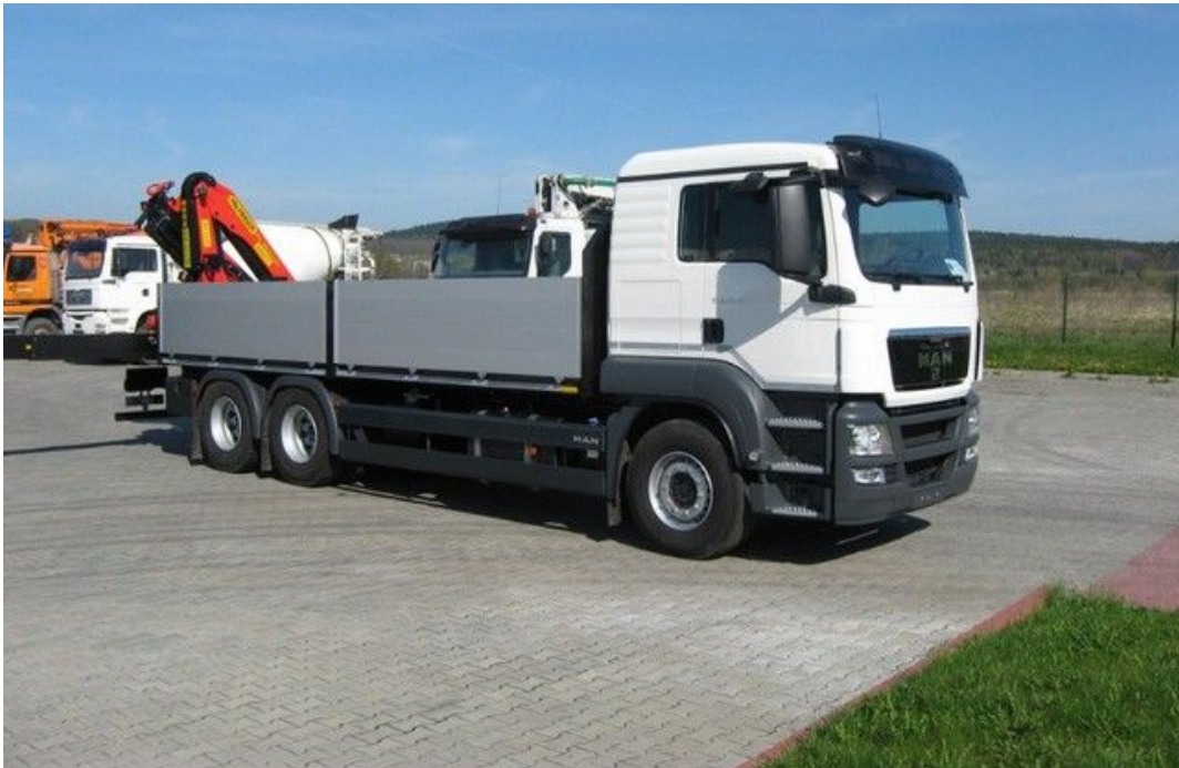
Obr. 7.54 MAN TGS 26.440 6x4 BL s HR PALFINGER 18001-EH [72]
