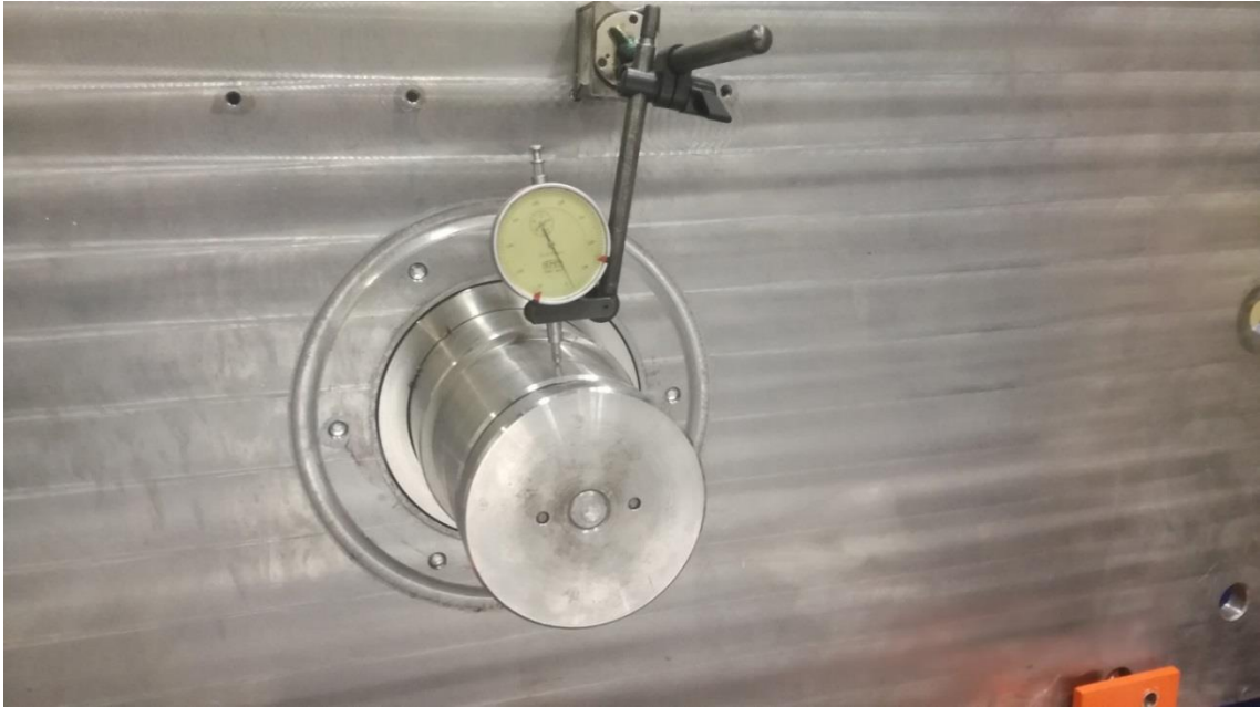
Fig. 9.8 Measurement of the sprocket shaft's deflection
