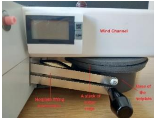
b. Showing outer rings were stacked on the base of the hotplate
