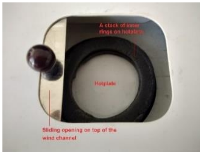
c. Showing inner rings were placed inside the wind channel on the hotplate
