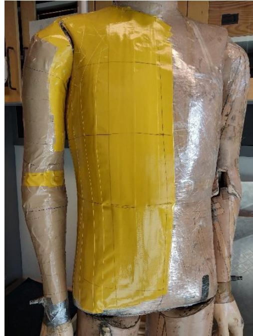
b. The molding method – duct tape was applied on top of the plastic shrink wrap, which was tightly wrapped around the torso of the manikin for protection and easy unmolding
