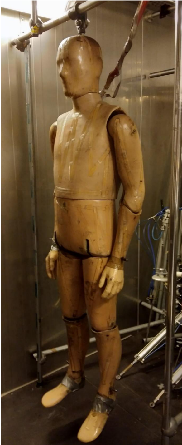
Figure 7. Tore- the dry manikin is in standing mode inside the climatic chamber
