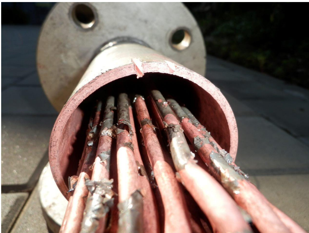
Figure 4.3 – Detail of spiral micro tubes with inner diameter 3.0 mm.
