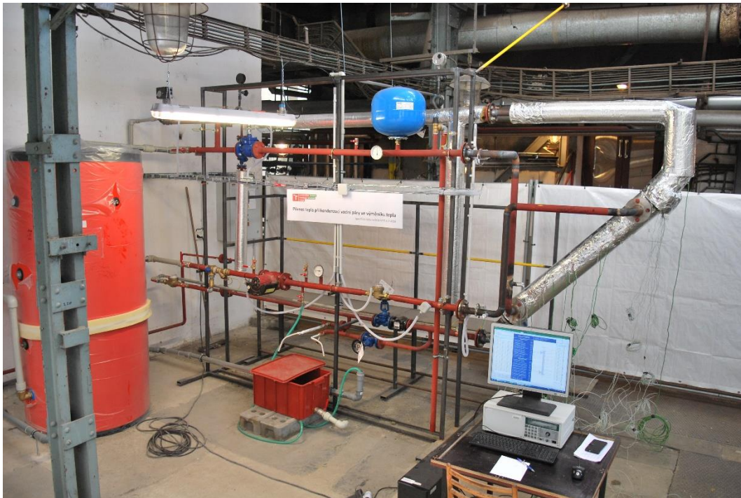
Figure 4.4 – Experimental setup of tubular heat exchanger.
