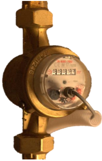
Figure 4.10 – Water meter G. GIOANOLA, IARC/25 R80, Class T90 with MaR recording system.
