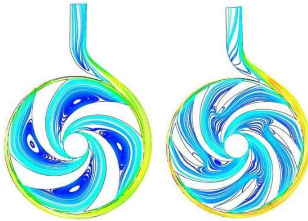
Fig. 5.79: Local eddies in the radial low specific speed pumps [34].
