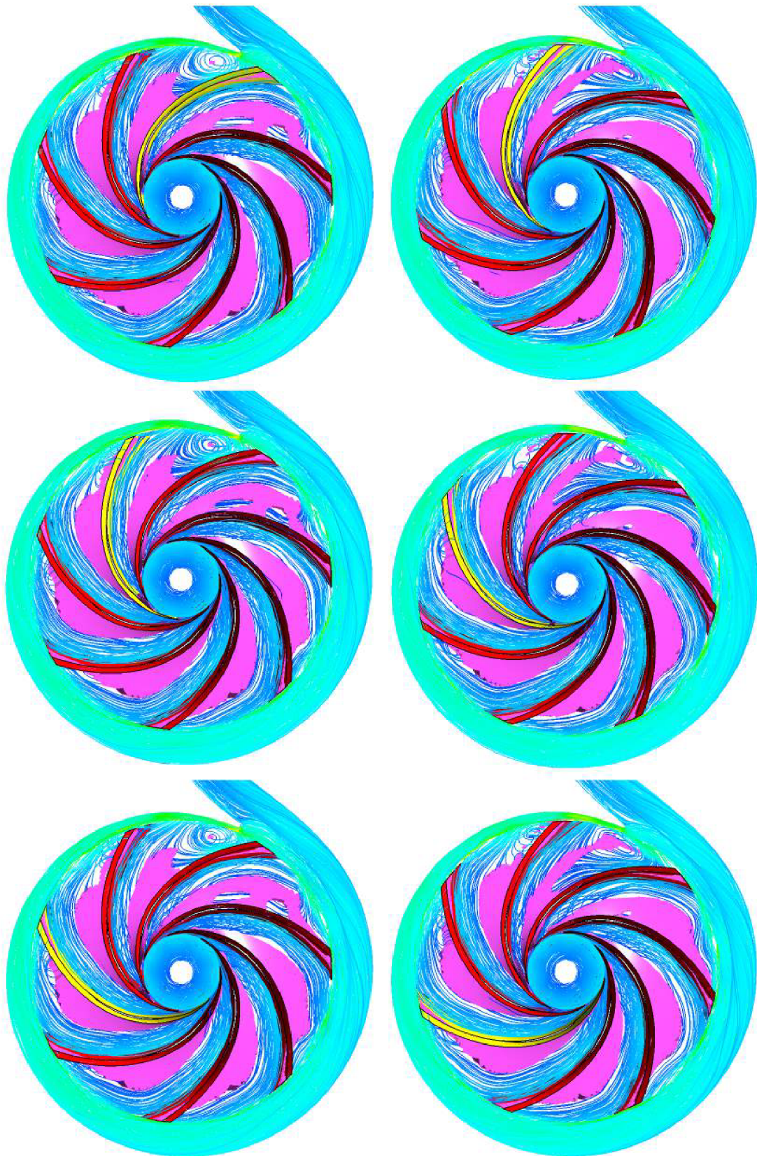
Fig. 5.108: Streamlines inside of the optimized impeller (optimal Q ).
