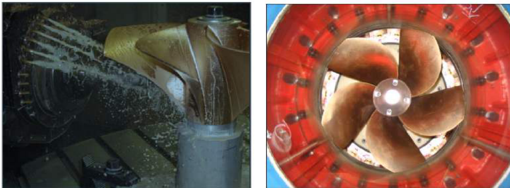
Fig. 1.10: CNC machining of "Mixer"(left), installation in the laboratory (right) [86].
