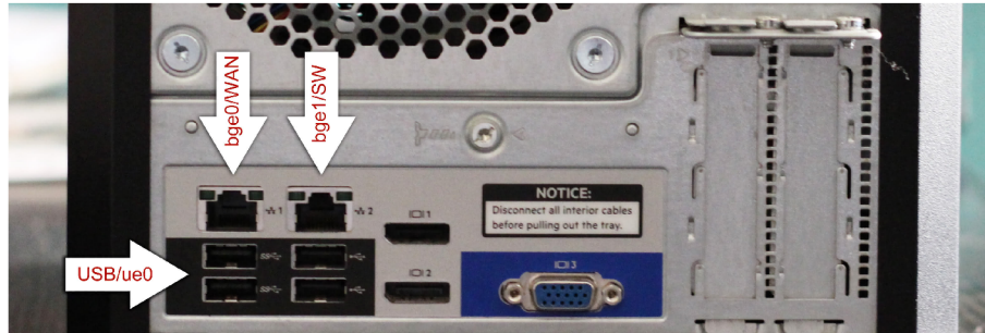
Obr. A.4: Zadní panel na HPE MicroServer Gen 10
