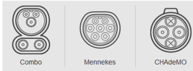
Figure 14: Different types of charging connectors for charging points
