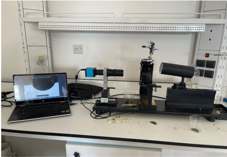
Figure 14 Schematic representation of a VIT-6000 apparatus used to measure IFT and contact angle.
