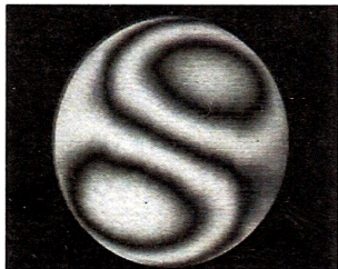
Figure 2.10: Interferogram at the cat's eye point
