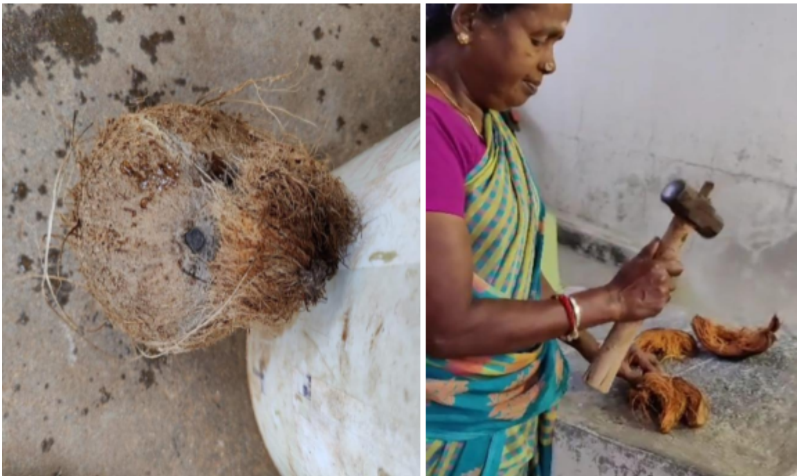
Fig 8. (a) Coconut after the removal of husk (b) Removal of fibers from husks
