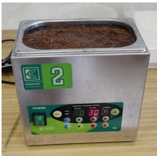
Fig 9. (a) Sonication of fibers
