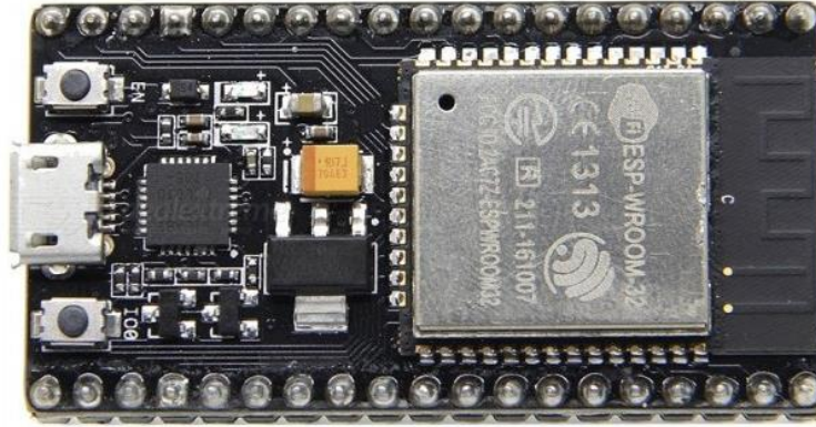
Figure 2.2: Node MCU ESP-32S with ESP32-WROOM-32 module soldered.[5]
