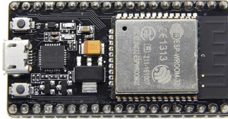
Figure 2.2: Node MCU ESP-32S with ESP32-WROOM-32 module soldered.[5]
