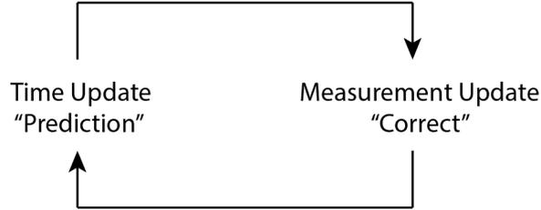
Fig. 6.2: Kalman filter iteration
