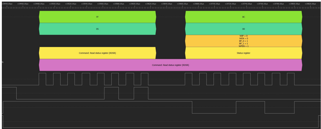
Figure 8.14: Rdsr command executed on emulator device
