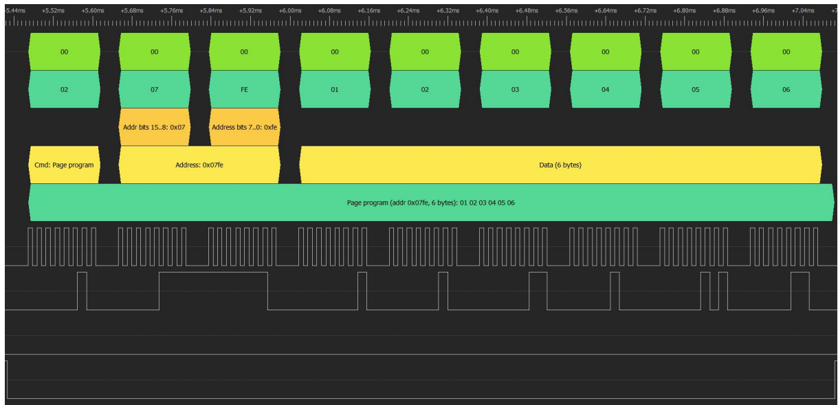
Figure 8.8: Write command executed on emulator device
