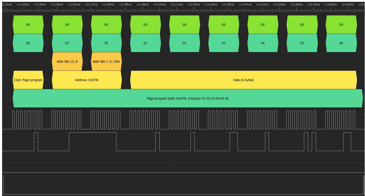
Figure 8.9: Write command executed on real device
