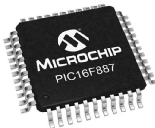
Figure 2.3: PIC16F887 microcontroller in 44TQFP package [6]
