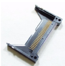
Obr. 3.7: Adaptér pro CF [35]
