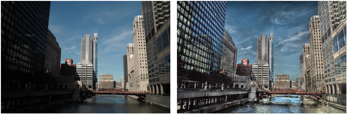
Figure 3.5: Left: Original image. Right: Output image processed by the method. Notable is brightening of dark area, where shift coefficients t_p shifted base layer to brighter values. Images are from authors' results [25].
