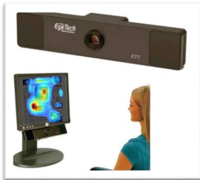
Figure 3 EyeTech's eye-tracking device attached to the participant's monitor displays
