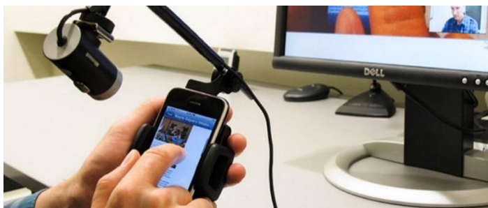
Figure 4 Camera for testing mobile devices .
