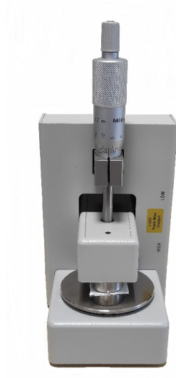
Obr. 7.2: Dielectric Test Fixture
