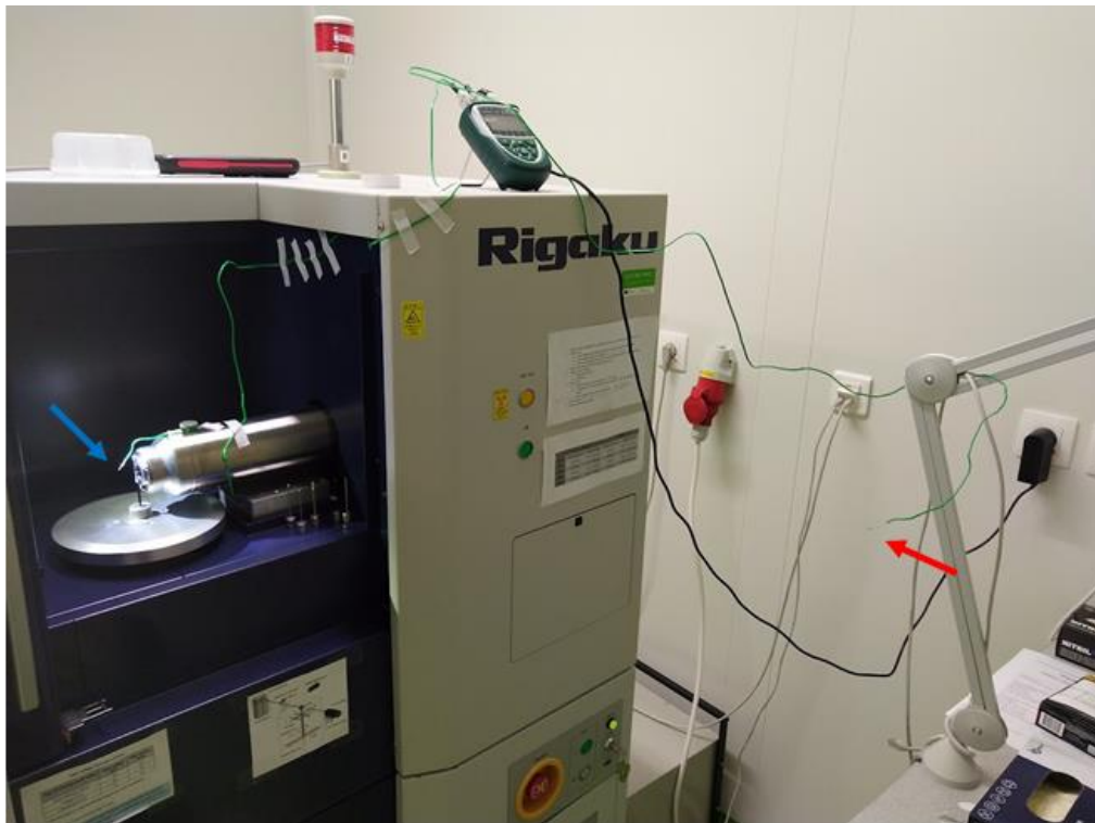
Figure 25: Arrangement used within the experiment – red arrow indicates sensor for measuring room temperature and blue arrow indicates sensor used for measuring chamber temperature.
